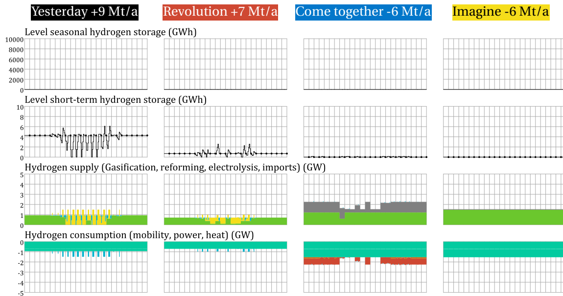
Figure 3.24: Hydrogen supply and consumption for a typical case of the four scenario variants: hydrogen storage , electrolysis , gas reforming , gasification , mobility , power , CHP , and heat
