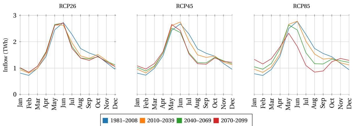
Figure 2.9: Inflows to run-of-river hydropower under different RCPs and climatic periods
