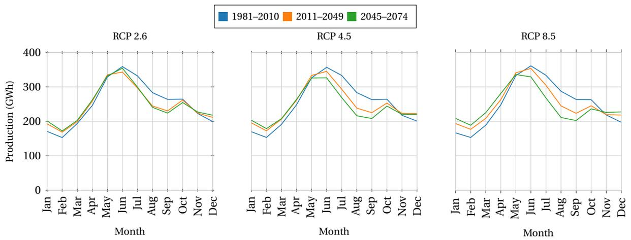
Figure 2.11: Hydropower production for Run-of-river (RoR) power plants in the CH2018 scenarios (CH2018, 2018, Wechsler and Stähli, 2019)
