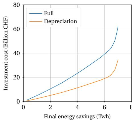
Figure 5.2: Energy efficiency cost curve for the Swiss commercial sector. From Streicher et al. (2020a)
