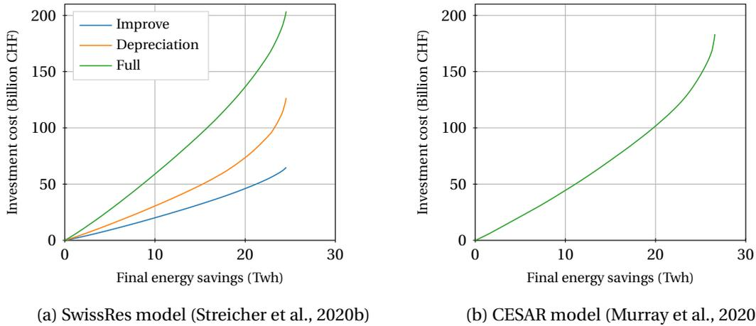
Figure 5.1: Energy efficiency cost curves for the Swiss building stock
